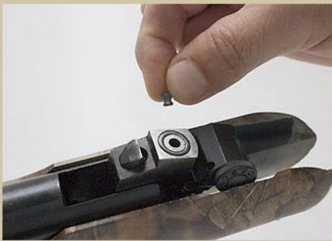
With the barrel in the broken open position, a .177-caliber pellet is simply inserted into the breech for loading.
